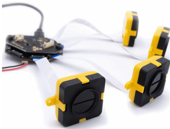
Figure 16 - Four TeraRanger Evo Mini sensors connected to Hub Evo
