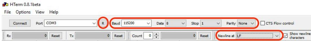
Figure 6 - HTerm parameters for TeraRanger Evo Mini
