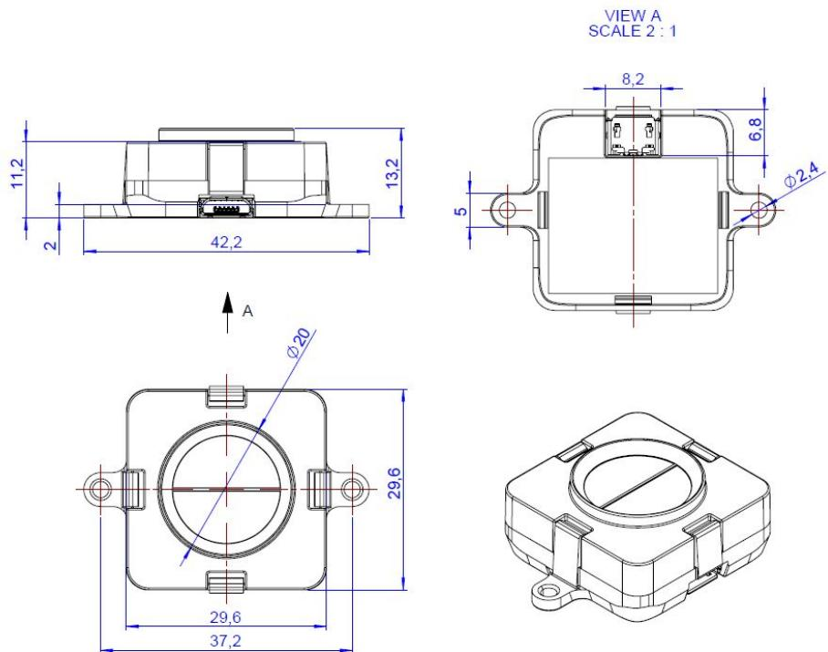
Figure 3 - TeraRanger Evo Mini external dimensions, USB backboard
