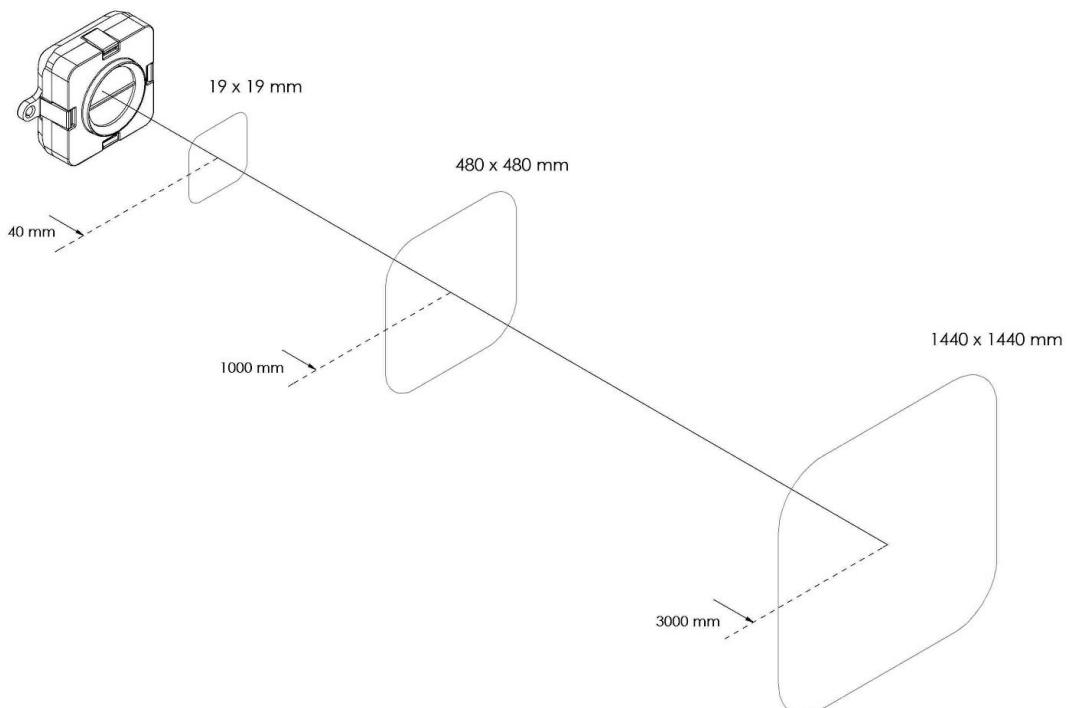
Figure 17 - Projected reception area for 1px mode.
