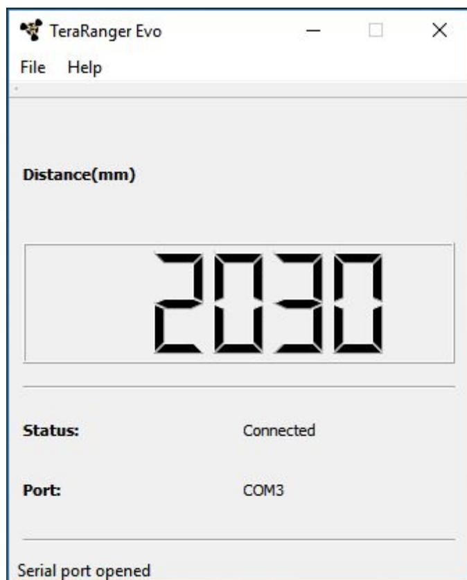
Figure 5 - TeraRanger Evo Mini GUI for 1px mode
