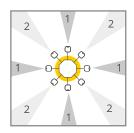
Sensors are activated 4 at a time, first odd port numbers, then even port numbers on the Hub Evo. This mode is best used for 360° environment monitoring.
