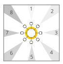
Sensors connected to the Hub Evo are activated one at a time (1 - 2 - 3 - etc). This mode is useful in configurations when crosstalk is likely and allows flexible sensor positioning.
