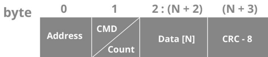
Figure 17. Frame structure for Evo Thermal commands
